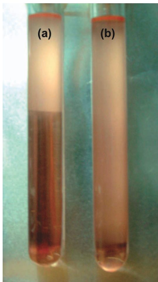
Figure 5 Molau test solutions consisting of 1,1,2,2-tetrachloroethane/phenol (4 : 6 by weight ratio) mixed solvents and the following blends: (a) PETG/uEVA (20 phr) and (b) PETG/mEVA (20 phr). [Color figure can be viewed in the online issue, which is available at wileyonlinelibrary.com .]
